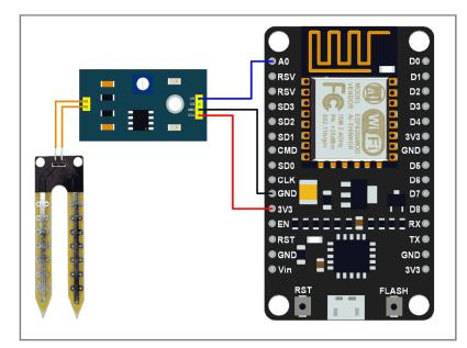
Here, the analog output of soil moisture sensor is processed using ADC. The moisture content in terms of percentage is displayed on the serial monitor. The output of the soil moisture sensor changes in the range of ADC value from 0 to 1023. This can be represented as moisture value in terms of percentage using formula given below.
