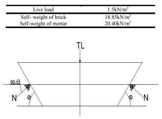
Figure 4. Forces on the system of bricks
