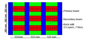
Figure 1a. Typical layout of ARS
