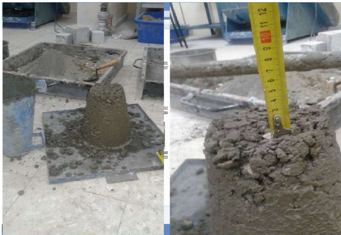
Figure 2. Slump test of concrete mix of 30% of OMW ash by weight of cement
