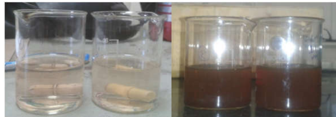
Fig.1. Green synthesis of Ag-nanoparticles– visible observation due to color change from transparent to brown
