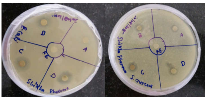
Fig.7. Antibacterial activity against E.coli (left) and S.aureus (right). (P.E) plant extract, (A) 25% Ag nanoparticles, (B) 50% Ag nanoparticles, (C) 75% Ag nanoparticles, (D) AgNO 3 solution
