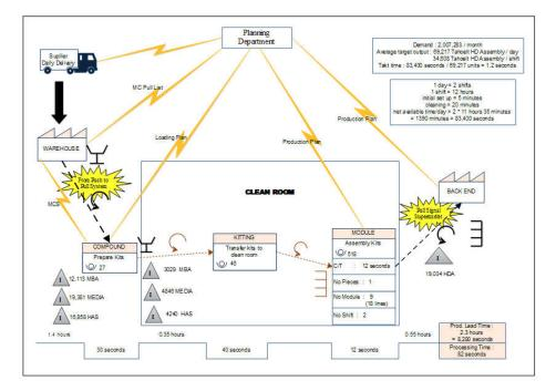
Fig. 4. Future State Value Stream Mapping
