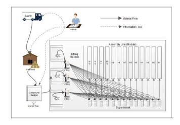
Fig. 1. The flow of material and information among supplier, Warehouse, Compound/Kitting section and Assembly line section
