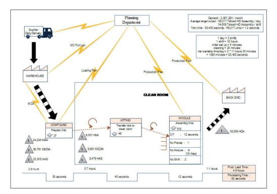
Fig. 3. Current State Value Stream Mapping
