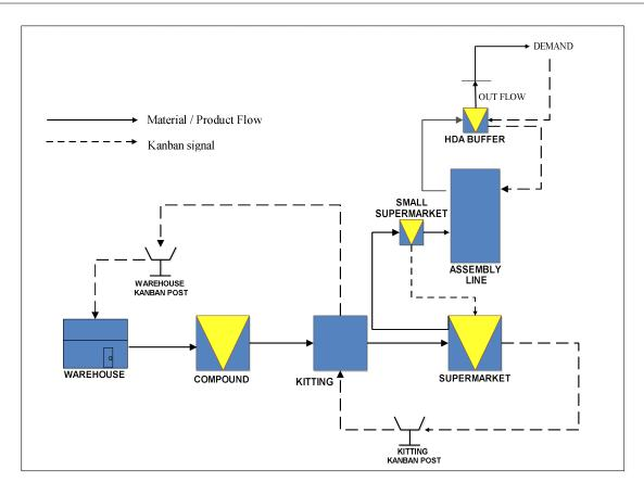
Fig 6. Material/Product flow for Simulation of Kanban System
