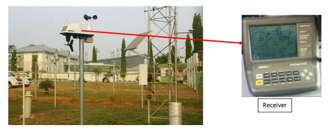
Figure 3. An Automatic weather station at the Abuja international Airport with sensors which measure pressure, wind speed and direction, dew point and humidity and displays the data/ weather information on the receiver to the right of the enclosure
