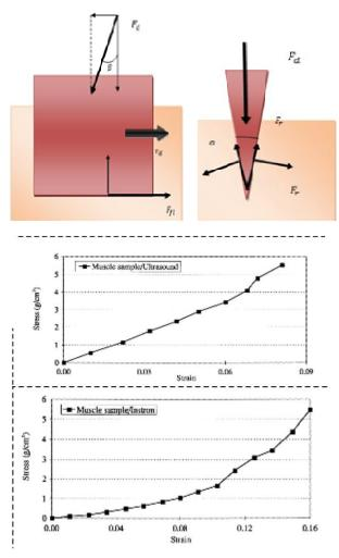
Graph 4, 5. The strain-stress curve for the liver tissue using both methods
