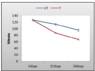
Figure 6: Effect on Nitrate content during vermifiltration of wastewater
