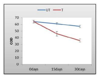
Figure 5: Changes in chemical oxygen demand (COD) during vermifiltration of wastewater
