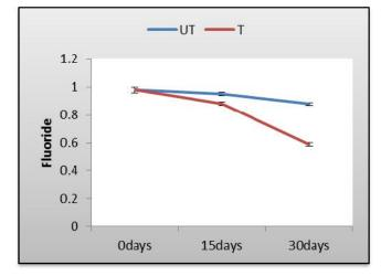
Figure 7: Effect on Fluoride content during vermifiltration of wastewater
