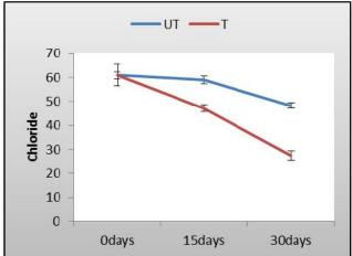
Figure 8: Effect on Chloride content during vermifiltration of wastewater
