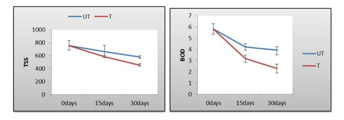
Figure 3: Effect of total suspended solids (TSS) during vermifiltration of wastewater
