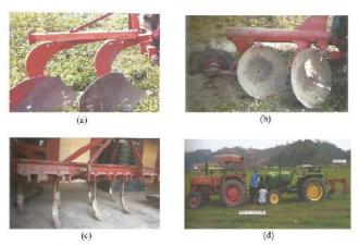
Figure 1 (a) 2 Bottom Mouldboard Plough (b) 2 Bottom Disk Plough (c) Spring Loaded 7 Tine Cultivator (d) Auxiliary Tractor (HMT) and Test Tractor (John Deer)
