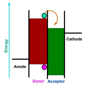
Figure 3. Energy levels and charge separation in an organic solar cell
