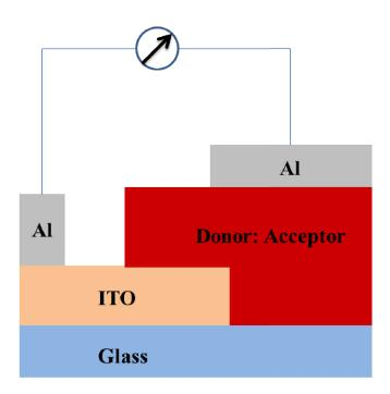
Figure 2. Schematic of the basic structure of a bulk hetero junction organic solar cell
