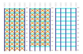
(a) Fully infilled frame (b) Soft storey with fully infilled frame (c) Bare frame
