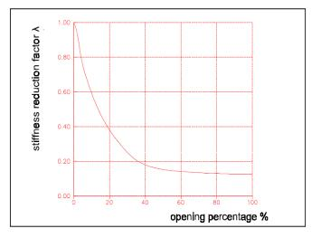
Fig. 4. Stiffness reduction factor 'λ' of the infilled frame in relation to the opening Percentage
