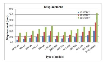
Fig. 6. Maximum displacement for 10, 15 and 20 storey building models in zone V
