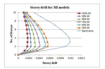
Fig. 8. Storey drift of 10 storey building for MIS and Bare frame models in zone V
