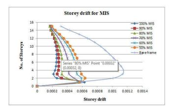
Fig. 11. Storey drift of 15 storey building for MIS and Bare frame models in zone V
