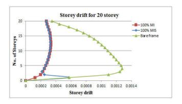
Fig.15. Storey drift of 20 storey building for fully infilled frame, soft storey and bare frame models in zone V
