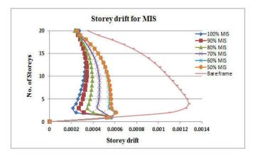
Fig. 14. Storey drift of 20 storey building for MIS and Bare frame models in zone V
