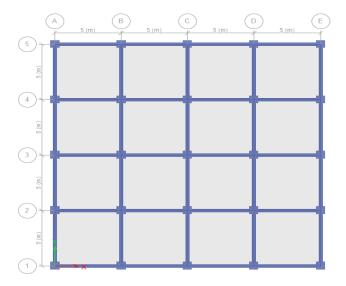
Fig. 2. Plan of 10, 15 and 20 storey building models
