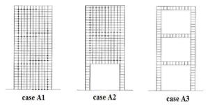
Fig. 1. Infill frames for three different cases of infill frame (P. G. Asteris, M.ASCE 2003)
