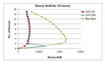
Fig. 12. Storey drift of 15 storey building for fully infilled frame, soft storey and bare frame models in zone V
