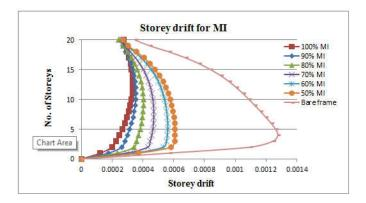
Fig.13. Storey drift of 20 storey building for MI and Bare frame models in zone V
