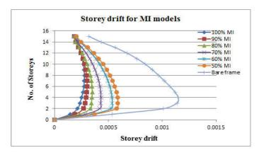
Fig. 10. Storey drift of 15 storey building for MI and Bare frame models in zone V
