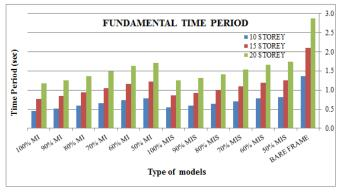
Fig. 5. Fundamental time period for 10, 15 and 20 storey building models
