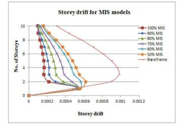
Fig. 9. Storey drift of 10 storey building for fully infilled frame, soft storey and bare frame models in zone V
