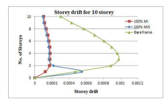
Fig. 7. Storey drift of 10 storey building for MI and Bare frame models in zone V
