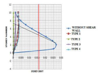
Fig. 7. Storey drift of building with and without shear wall by push over analysis
