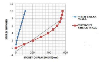
Fig. 7. Storey displacement of building with and without shear wall by using push over analysis
