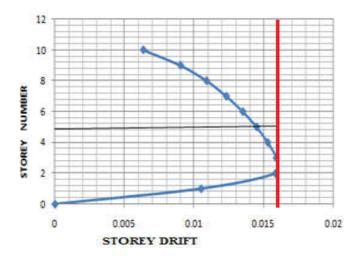
Fig. 6. Storey drift of building without shear wall by linear response spectrum analysis
