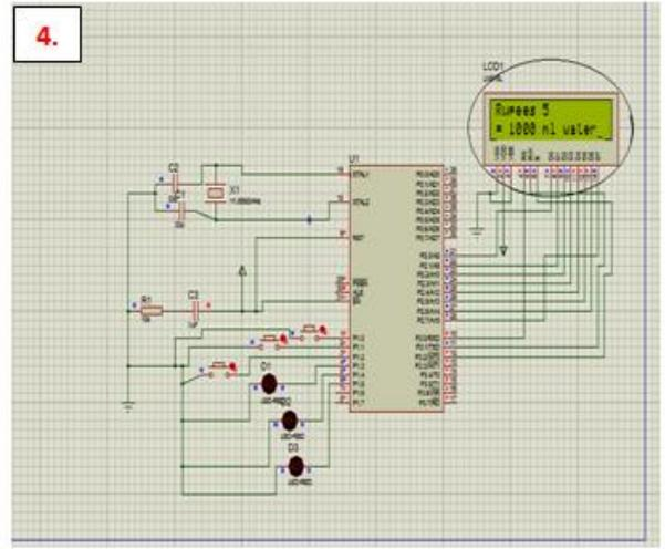
Fig.9. In this the LCD will display the amount and respective quantity of water. For Rs.5 it will give 1000ml water
