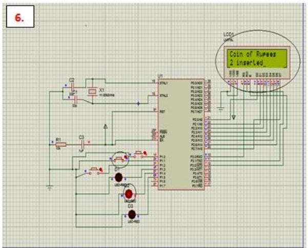
Fig.11-In this the LCD will display the message after the coin of Rs. 2 is inserted. Here encircled switch is considered as input for Rs.2.
