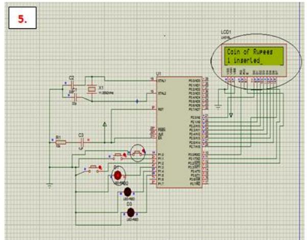
Fig.10. In this the LCD will display the message after the coin of Rs. 1 is inserted. Here encircled switch is considered as input for Rs.1.
