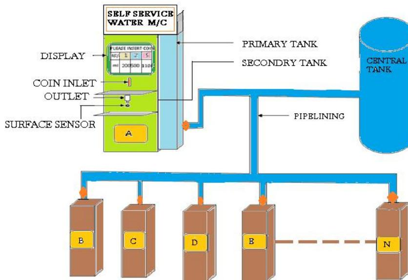
**Fig.5. Work flow diagram**
