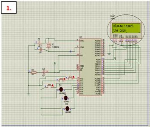
Fig. 6-At the initial stage the LCD will continuously and display the message “Please insert the coin”
