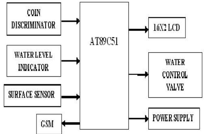
**Fig.2. Block Representation of proposed system**
