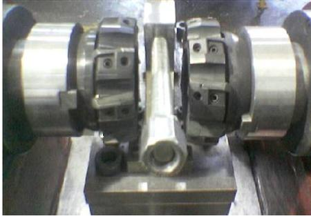
Fig. 8. Duplex milling machine
