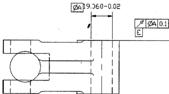
Fig. 4. shaft hole boring
