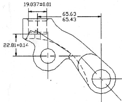
Fig. 6. Socket bore drilling
