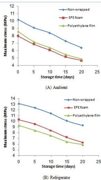
**Figure 3. Maximum stress versus storage time at two different storage conditions**
