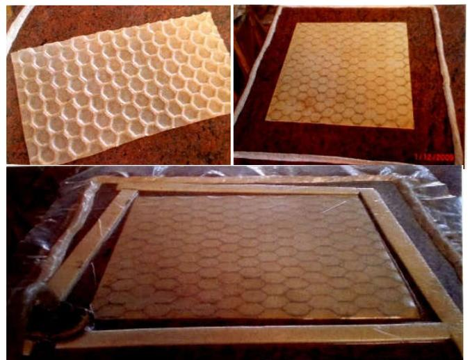
Figure 4. Fabrication of honeycomb sandwich panel
