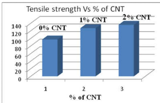
**Graph 1. Tensile Strength (N/mm2) Vs % of CNT**
