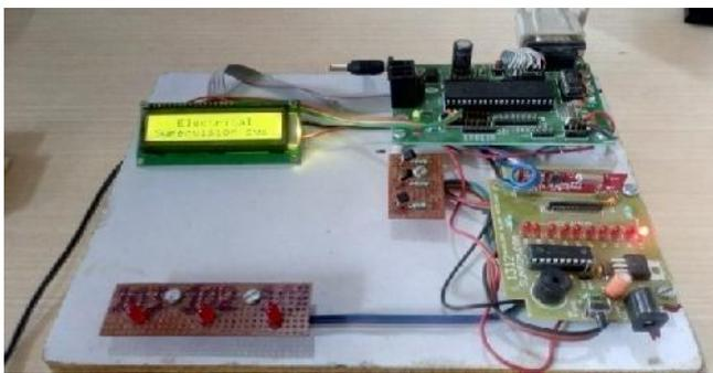
Figure 3. Experimental Setup for RFID Based Electrical Supervisor
